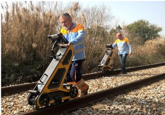
Continuous Inspection with Portable Equipment
